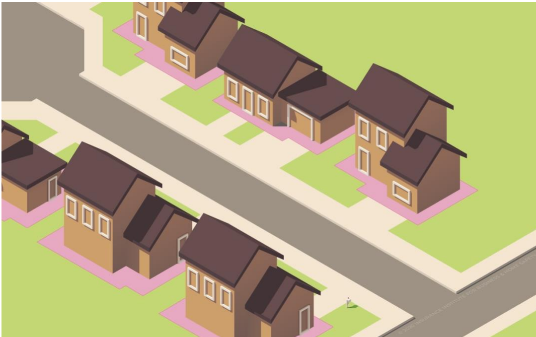
Figure 1. View of a typical suburban street and cul-de-sac highlighting in pink the 0–5 ft noncombustible zone.
