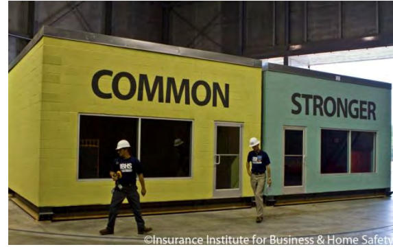
The two test specimens above were used in the first full-scale high-wind test of commercial structures at the IBHS Research Center.
