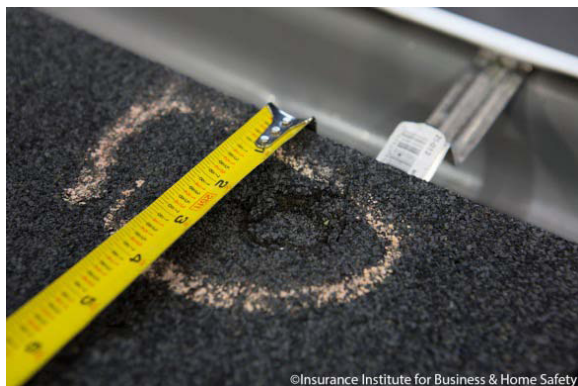
Damage is shown to a 3-tab shingle on the test specimen. The majority of impacts on these shingles were severe enough to be considered functional damage.
